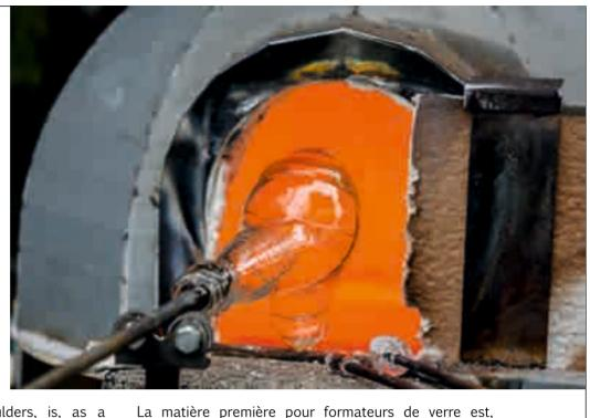
The raw material for glass moulders, is, as a general rule, silicon dioxide in the form of sand. Glass is composed of about ¾ of silicon dioxide and other substances which reduce the fusing temperature, the hardness, the colouring or the de-colouring of the respective glass. Potassium (plant extracts) is necessary to guarantee the required flow (to reduce the temperature of fusing). Plaster is necessary for the hardening of the glass. To colour and de-colour the glass, oxides are needed.
