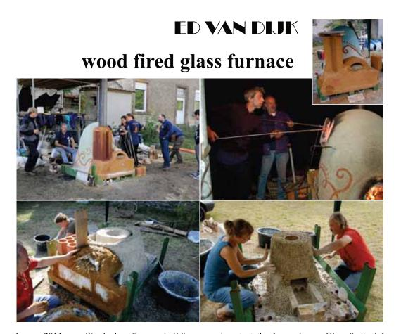
In my 2011 woodfired glass-furnace building experiment at the Luxembourg Glass-festival I decided not to use any firebrick for building the furnace. The wood-fired glass-furnace I build in Belgium in 2010 was out of firebrick. But building with locally found materials ,like clay and stone, would be much closer to glass-furnace building in ancient times.
